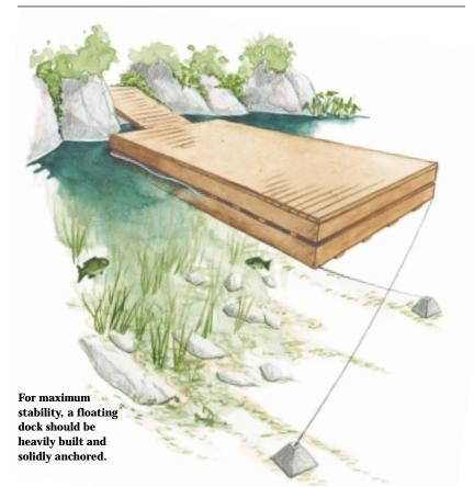
wide, low, and heavy. The consensus among dock builders is that  $6' \times 20'$  is the minimum size for a stable floater, this single section weighing in at about 1,000 lbs, minimum. And bigger is even better.
